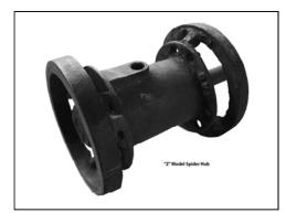
The Cottonreel Hub is the most common and is the latest of the models. This hub was also used for a time on the "IZ" Model when it was first released. The Wheel Arms are bolted to the flanges at the front and the back of the Hub, and retained using Cast Clamps and "U" Bolts. The Spider Hub was changed to the Cotton Reel Hub is about 1944
