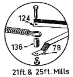
Method of Connecting Check Chain to Bracket.
